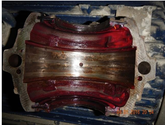
Gambar 11 Kondisi Housing Bearing
