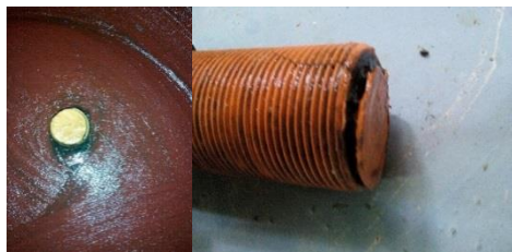
Gambar 4. 2 Sensor speed switch tergerus metal target
